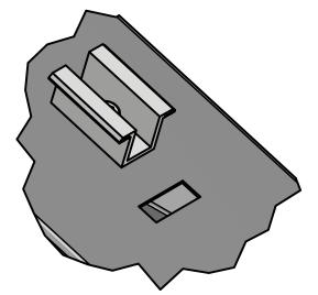
In the next step, we attach the clamps to the triangles, for this purpose we use allenscrews and tighten them with flange nuts. It should be remembered that they are not tightly tightened due to the need to adjust to the modules. As an alternative, basket nuts can be used. They replace the aluminum keyway.
