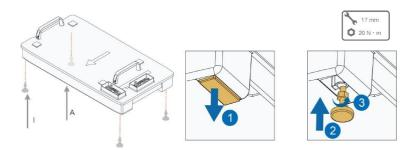
2. Place the base at the acceptable position in right way (arrows outward).
