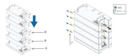
4. Insert BMU (make sure the DC MCB is off) and screw.
